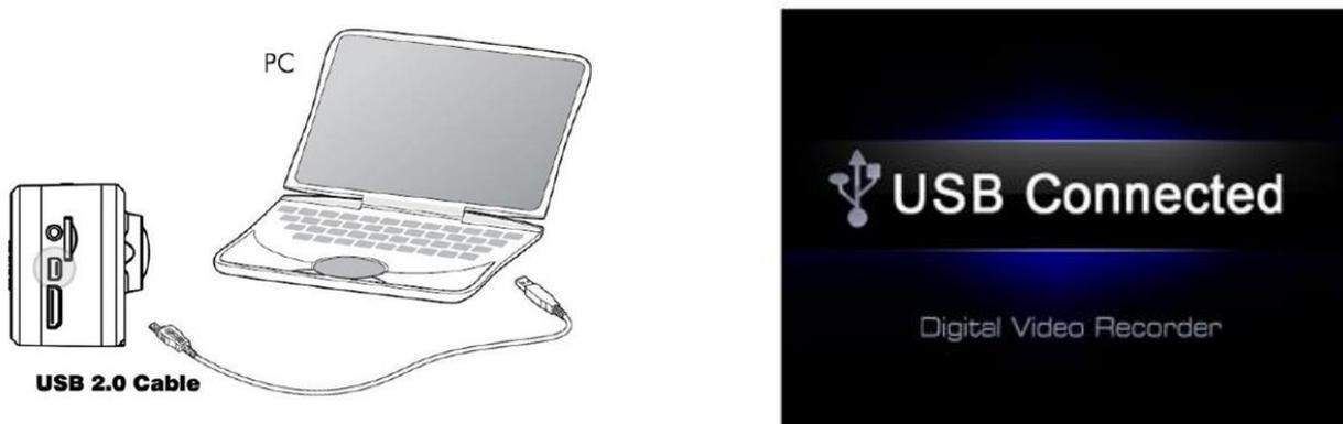
**Important Note:** When connected to a PC via USB all features **will not work** directly from camera, such as Record, Playback and Browse. Charging the battery will occur as well as data transfer via the connecting computer only.
