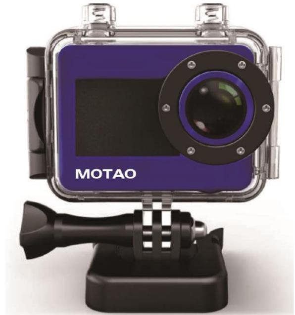
**Note!** Your camera mounts are rugged but they are plastic and may break under heavy stress and certain rough riding conditions therefore it is recommended that you tie a thin tether line to the camera housing. If the camera should break lose during riding it will remain tethered to the bike. Make sure the tether does not connect to or near moving parts of the motorcycle.
